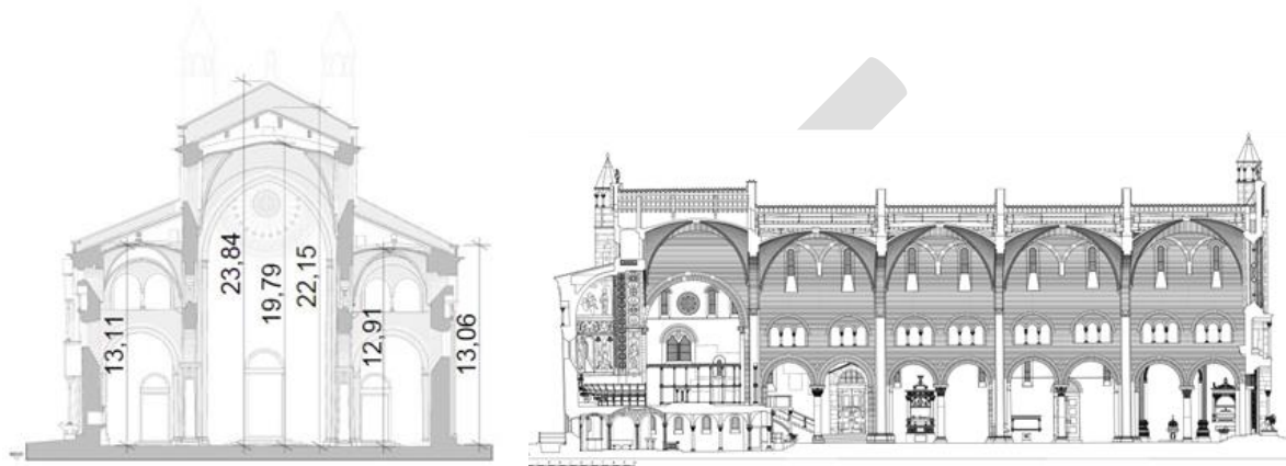
Figure 5: Cross-section of the Cathedral of Modena
