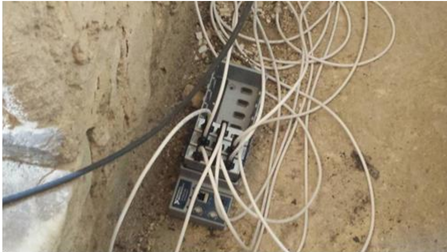
FIGURE 29 – CHASSIS MODULE NI9188 WITH 8 SLOTS FOR DAQ CARD.
