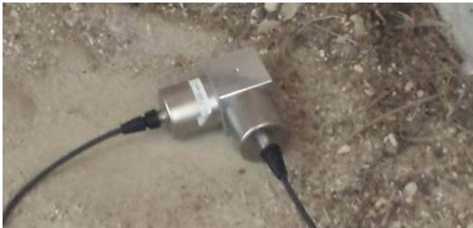
FIGURE 30 PIEZOELECTRIC ACCELEROMETERS PBC OF THE NATIONAL INSTRUMENTS, ORTHOGONAL BETWEEN THEM.
