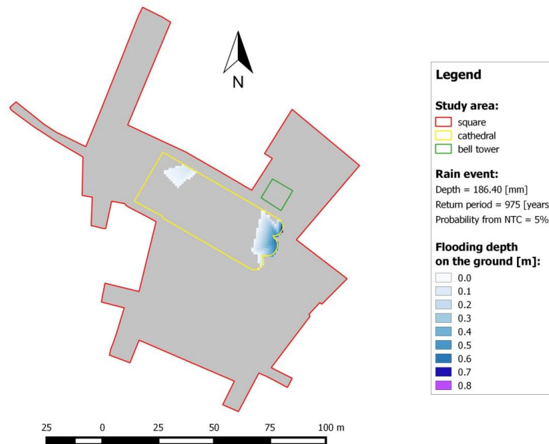
Figure 2.1.29 - Maximum flooding depth on the ground for a precipitation depth equal to 186.40 mm.
