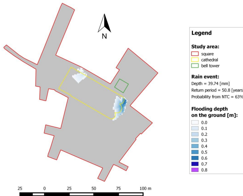
Figure 2.1.22- Maximum flooding depth on the ground for a precipitation depth equal to 39.74 mm.
