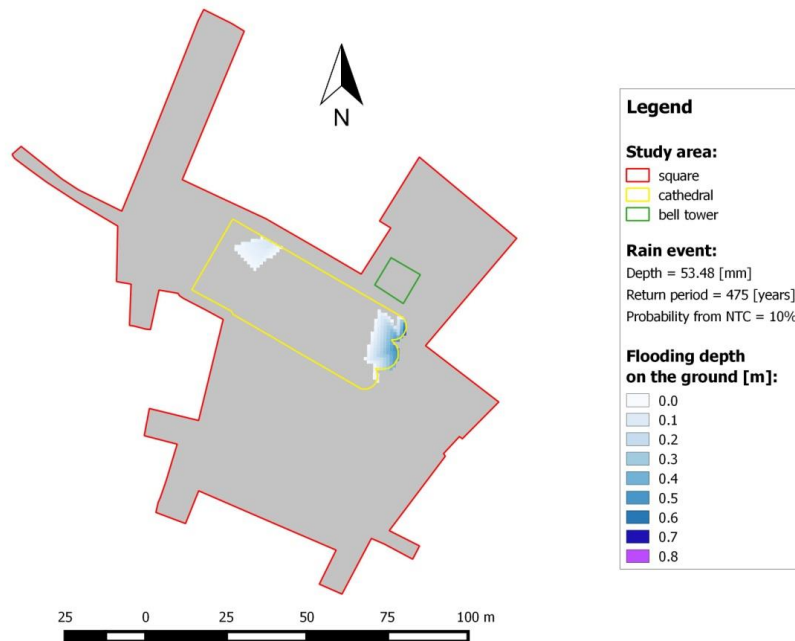
Figure 2.1.28 - Maximum flooding depth on the ground for a precipitation depth equal to 53.48 mm.
