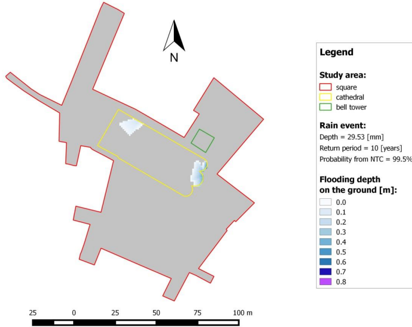
Figure 2.1.25 - Maximum flooding depth on the ground for a precipitation depth equal to 29.53 mm.
