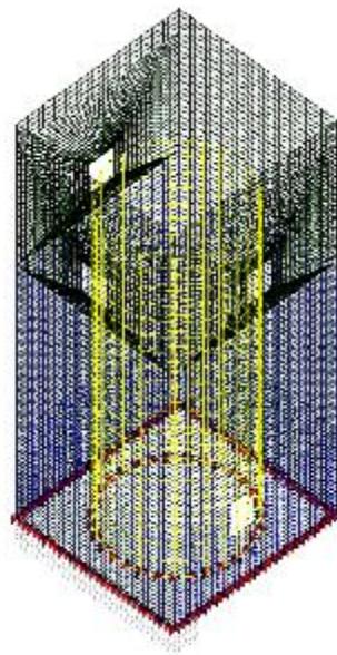
FIGURE 66–PROSAP FE-MODEL OF THE TOWER WITH IMPOSED VERTICAL DISPLACEMENT
